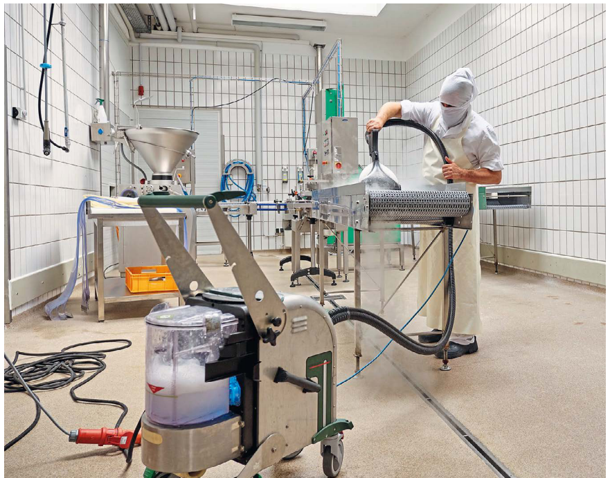
The Göschle truffle manufactory thoroughly rids the most diverse surfaces of dirt, germs and bacteria – solely with dry steam.
