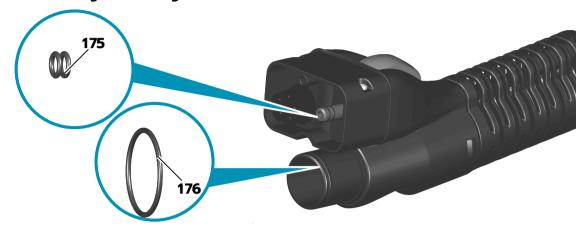
Figure 4.4-3 Change the O-rings on the suction and steam hose
