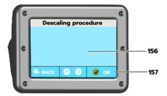
Figure 4.3-4 Start the descaling programme
